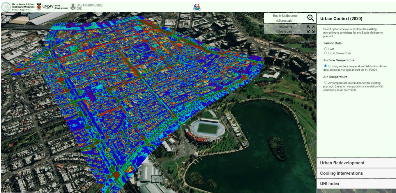
Figure 42: Surface temperature distribution of the existing urban conditions in the South Melbourne Study Area
