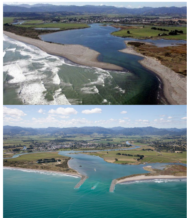
Figure 1: Existing Waioeka River entrance and proposed including river training works (source: ODC|stuff.co.nz)
