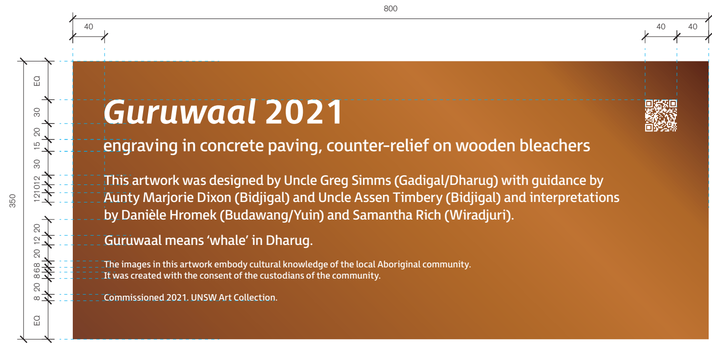
03 Detail Scale 1:4 Spec Artwork plaque to be 3mm thk aluminium with Astor Metals Arcturus aged bronze satin finish (or similar). All messaging as white digital print direct to panel surface. Contractor to ensure longevity of digital print in outdoor conditions and ensure no fading or blurring.
